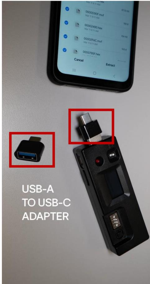
② After connecting the JIG and the smartphone, turn the JIG power ON.
