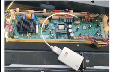
2. Please connect the connector to the refrigerator's Main PCB.
