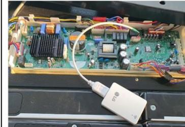
2. Please connect the connector to the refrigerator's Main PCB.
