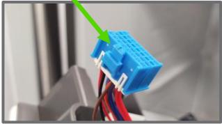
\*\*Note: The release tab is located on the left side of the connector and in some cases, there is not much room to get your finger on the tab to press it. In that case use a short flat blade screwdriver to press in on the tab so it will release from the connector:
