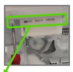
\*\*Note: Make sure once Icemaker is reinstalled that there are no gaps between the icemaker and freezer liner. Should be fully flush to liner on the sides and across the front\*\*
